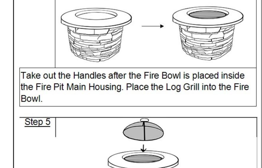
Put the Spark Safeguard Screen onto the top opening of the Fire Pit Body and make sure it sits into it evenly. The Firepit is ready for use.
