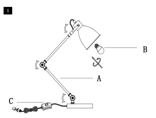
Step 1 Put the lamp (A)on the table . Insert the bulb(B)into the socket . push the switch(C)to make light.
