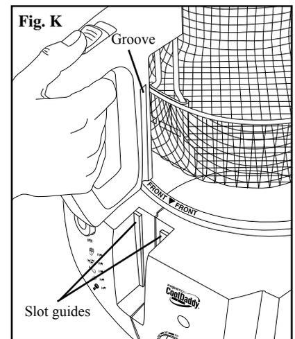
7. When frying time has elapsed, lift up on the basket handle to raise the basket to the drain position.
