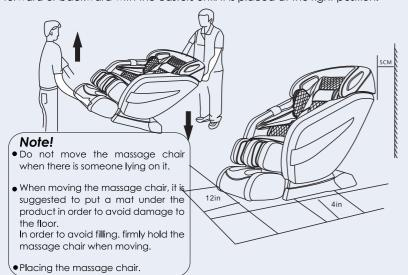
When placing the massage chair, leave enough space around the chair so that the leg and back of the chair can be lifted up and down freely. It is suggested to place the massage chair as shown in the right figure.
