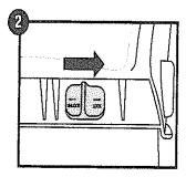
Move both sliding locks to the "LOCK" position. Slide both to the "UNLOCK" position anytime you want to fold up and store your Portable Pet Steps.
