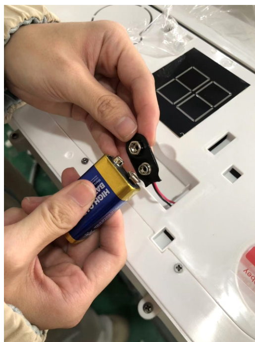
Step 2 Connect the battery.
