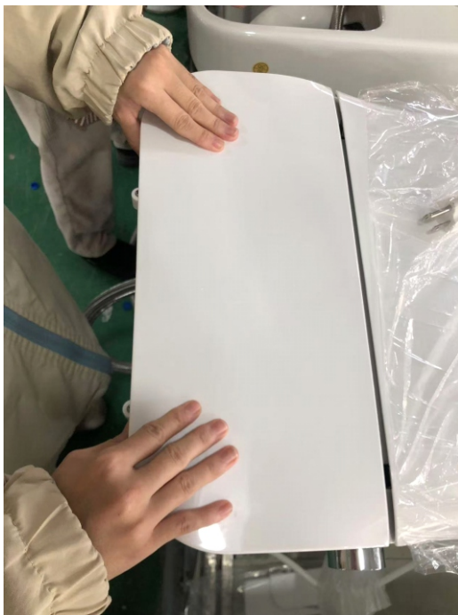
Step 1 Slide the back cover to open it.
