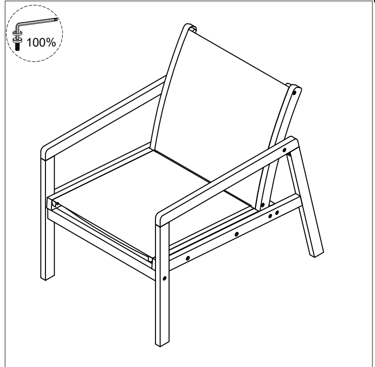
Step 6: Put the Chair upright and make sure all legs are level, then firmly tighten Bolts with Allen Key (4)
