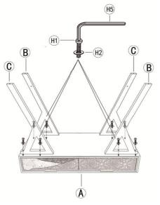
Step 2: Place the Shelf (D) to the Legs (B&C) with Hex bolt(H3)by Allen key (H5) as below photo shown.
