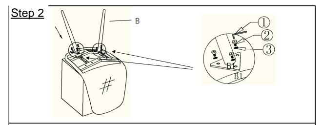
Align the Front Legs(B) with the mounting positions on the base of the Seat(A).
