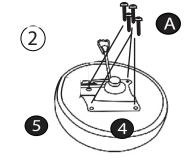
2.Insert A Screw × 4 into the hole of the 4 into the 5.
