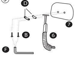
3.Insert B Screw × 2 into the D into the 6 into the 5 and hand tighten.
