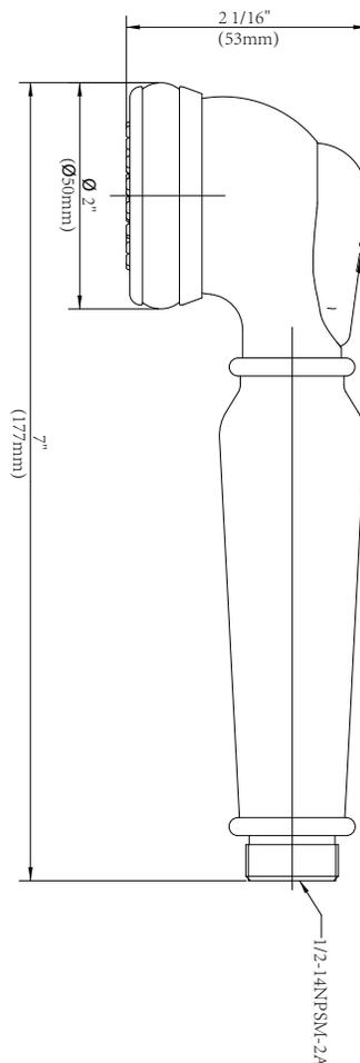
\* Danze Soft Touch Personal Shower is designed to operate only when the button is pressed; water will flow to the spout whenever pressure is released from the button.
