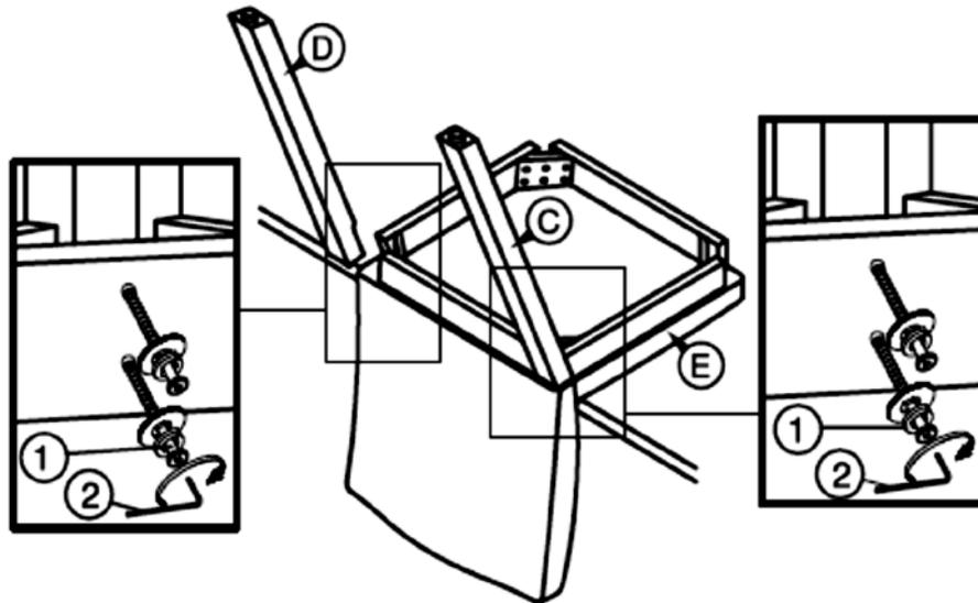
Place the Cushion Chair **Seat**(E) on the clean Table Top and place the Back Leg (C) Back Leg (D) on the corner block as shown.
