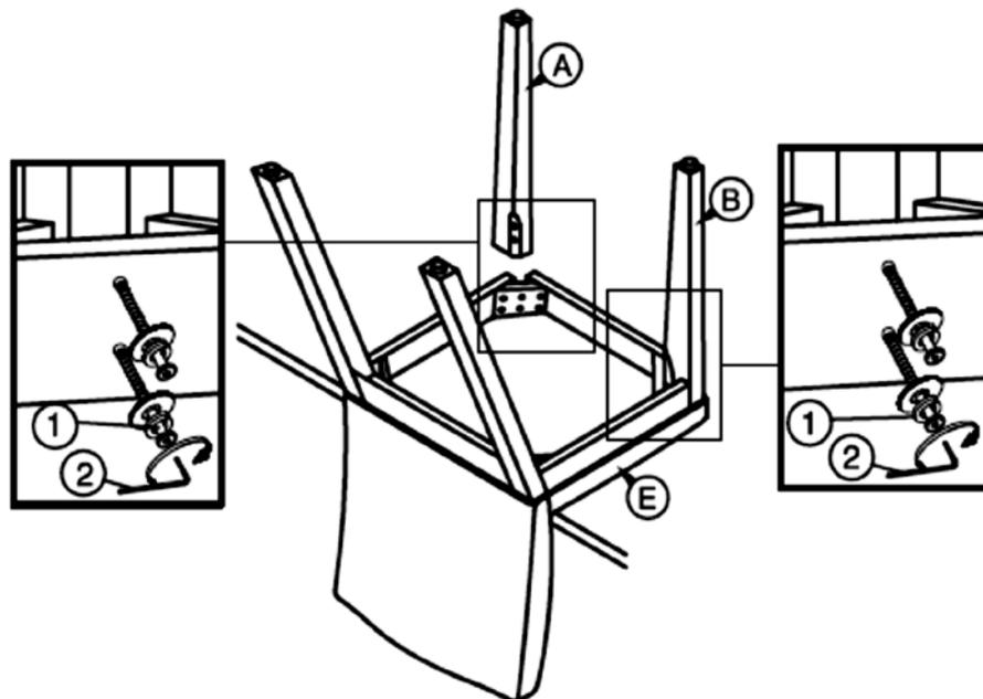
Repeat Step 1, place the Front Leg (A) and Front Leg (B) on the corner block as shown.
