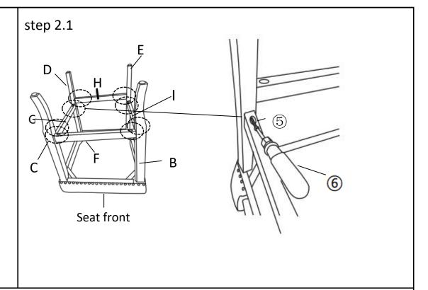
2.1 Insert the Side Rail (G) into round housing of the Legs (D) as shown above.
