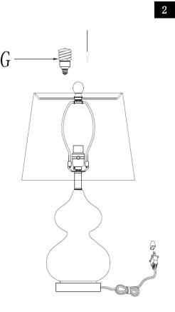
Step2 Insert the bulb(G) into the socket(C).
