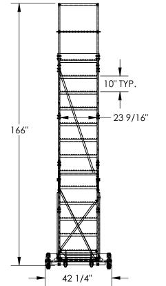
STANDARD FEATURES MODEL NUMBER IS LAD-13-14-G OVERALL WIDTH IS 42 1/4" USABLE WIDTH IS 23 9/16" **OVERALL LENGTH IS 95 9/16" USABLE LENGTH IS 91 5/16" OVERALL HEIGHT IS 166"** TOP STEP HEIGHT IS 130" STEP TYPE IS GRIP STRUT CLIMB ANGLE IS 58° STEP DEPTH IS 7" TOP STEP DEPTH IS 14" MAX CAPACITY IS 350 LBS WHEEL SIZE IS Ø10"
