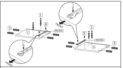
**STEP9**: Insert Dowel Medium (HW3) into Side Board Left (C) and Side Board Right (D).
