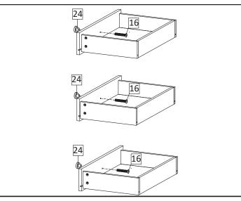
**STEP4**: Use Screw M4x22mm (HW16) to attach Handle (HW24) to the Front Drawer.
