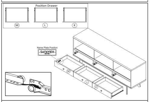
**STEP24**: Hold the sides of drawer, position the wheel of rail at drawer back and the wheel of rail at side boards, according to the image. Slide in the drawers one by one into the Media Stand.
