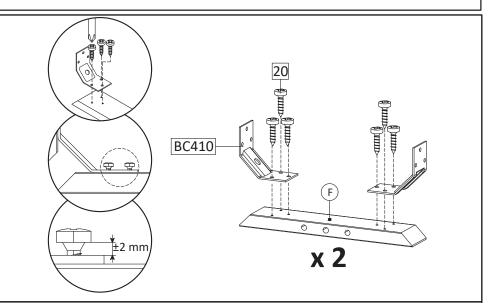
**STEP16**: Now let's combine the bottom skirt. Start with installing Corner Brace (HW BC410) into Support Leg 2 (F) using Screw M4x16mm (HW20).Do not overtight screw yet, leave around 2mm gap.
