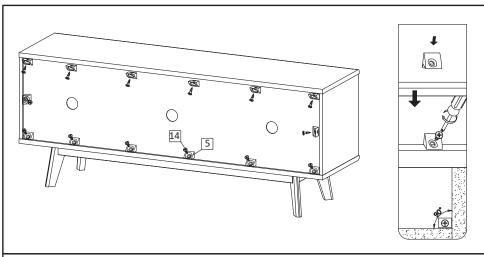
**STEP27**: Use Wedge (HW5), Screw M 3.5 x15.5 (HW14) to tighten the back of Media Stand by using screwdriver. Please align the top board and bottom board in  $90^{\circ}$  position against the side board, before securing the wedges (HW5).
