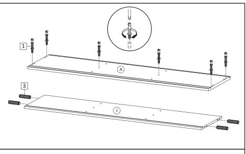
**STEP8**: Insert Cambolt (HW1)into Top Board (A). Insert Dowel Middle (HW3) into Fixed Shelf (J).
