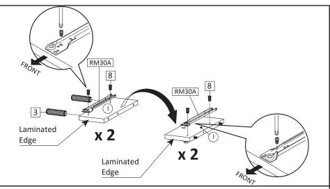
**STEP10**: Part of Metal Runner must be installed to Center Board small (I) on both sides. Secure part of the metal runner (HW RM30A) into position as the above image, using screw M6x10.5mm (HW8), then flip the board to access the opposite surface, continue to secure part of metal runner (HW RM30A) using screw M6x10,5mm (HW8).
