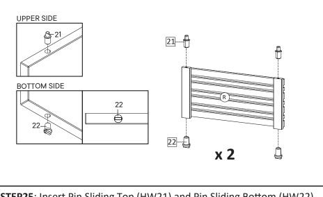
**STEP25**: Insert Pin Sliding Top (HW21) and Pin Sliding Bottom (HW22) on both end of frame door as specified position in the figure.
