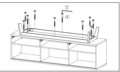
**STEP22**: Insert Screw M6.4x53mm (HW4) into position. tighten screws using Allen Key (HW7).
