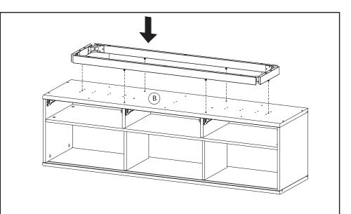
**STEP20**: Bring the assembled bottom skirt and insert into Bottom Board of the Media Stand.
