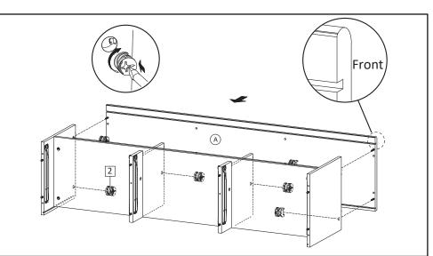
**STEP14**: Bring the Top Board (A) into assembled component. Secure with Camlock Big (HW2) and tighten it using screwdriver.
