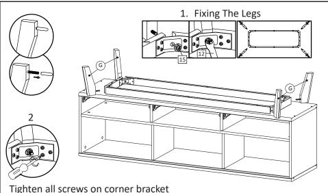
**STEP21**: Remove plastic cap from Legs. Insert the bolt of the Leg (G) into hole of
