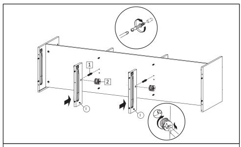
**STEP13**: Attach Center Board small (I) into the assembled component from step 12. Insert Cambolt (HW1), Camlock Big (HW2) and tighten it using screwdriver.
