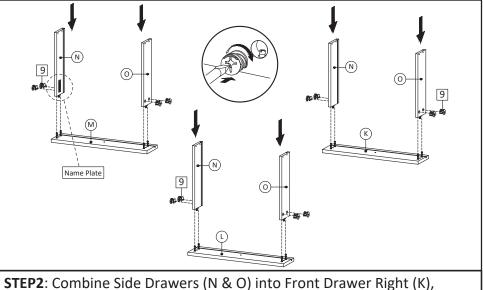
**STEP2**: Combine Side Drawers (N & O) into Front Drawer Right (K) Front Drawer Middle (L) and Front Drawer Left (M) then tighten camlock (HW9) using screwdriver.
