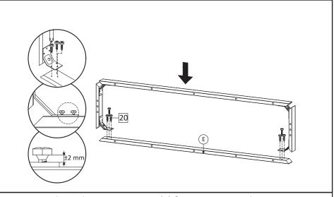
**STEP18**: Combine the Support Leg 2(F) from step 17 with remaining Support Leg 1 (E), using Screw M4x16mm (HW20). Do not overtight screw yet, leave around 2mm gap.
