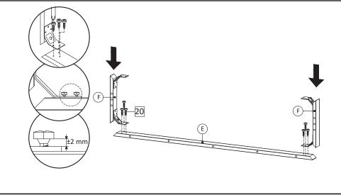
**STEP17**: Combine components from step 16 with remaining Support Leg 1 (E), using Screw M4x16mm (HW20). Do not overtight screw yet,leave around 2mm gap.
