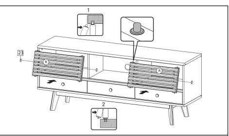
**STEP26**: Peel the back paper of Bumper (HW23) then 2 pcs on Frame Door Left, 1 pc on Frame Door Right, position as shown in the figure.
