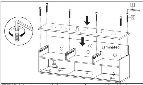
**STEP15**: Bring the assembled components from step 14 upside down with the Top Board on the floor. Insert Back Board (S) into position. Then put Bottom Board , secure with Screw M7x50mm (HW6) , tighten screws using Allen Key (HW7). Put the Screw Cup (HW11) over the tightened camlock.
