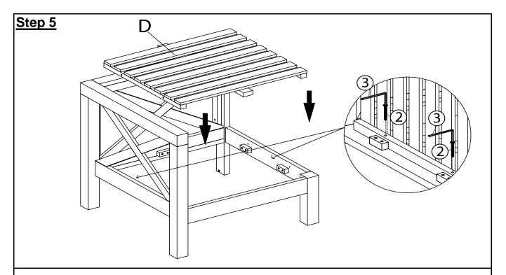
Attach the Seat Panel (D) into the Chair as shown in picture above.
