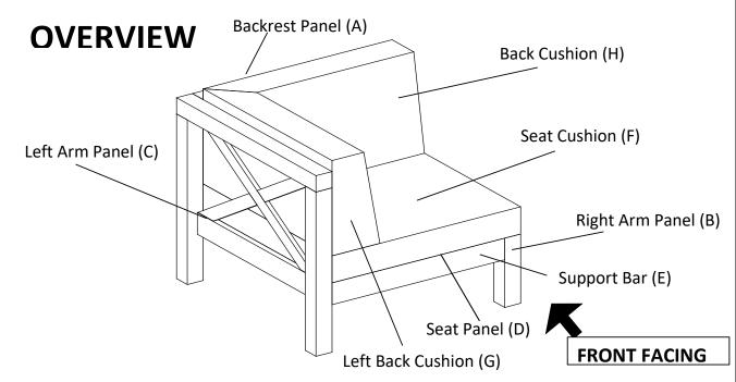
This Left Chair has multiple parts and may require up to 30 minutes to assemble. To give you an overview of the Left Chair parts, the above picture is to help you put the various parts into perspective. Please read through the instructions herebelow to familiarise the parts and steps before assembly.
