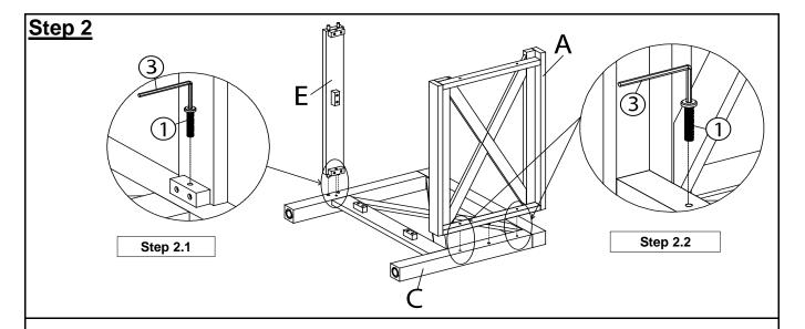
Place the Left Arm Panel (C) with inside face skywards onto a clean, soft surface to avoid any scratches or damages to the product.
