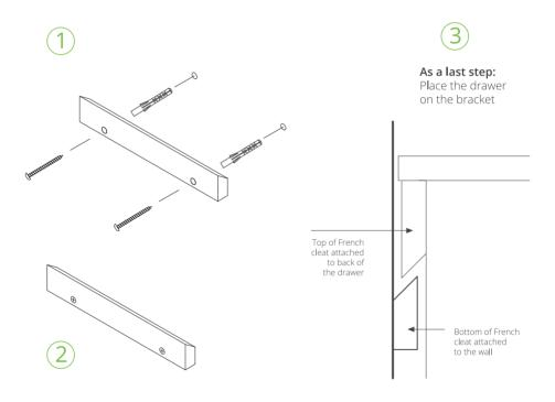
**Wall fixings:** As wall materials vary, screws for fixing to wall are not included. For advice on suitable screw systems, contact your local specialised dealer.
