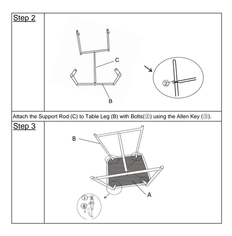
Attach Table Leg (B) to Table Top (A) with Bolts((1)) and Washers ((4)) using the Allen Key ((3)).
