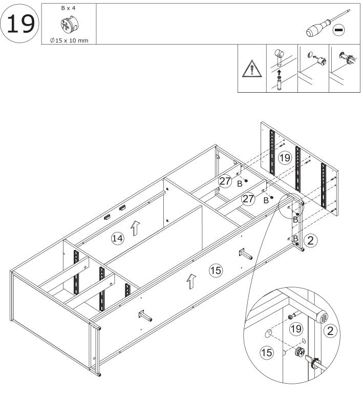
Attach board 19 to board 15 and 27, add cam lock(B) into board 15,27, turn clockwise to tighten as shown.
