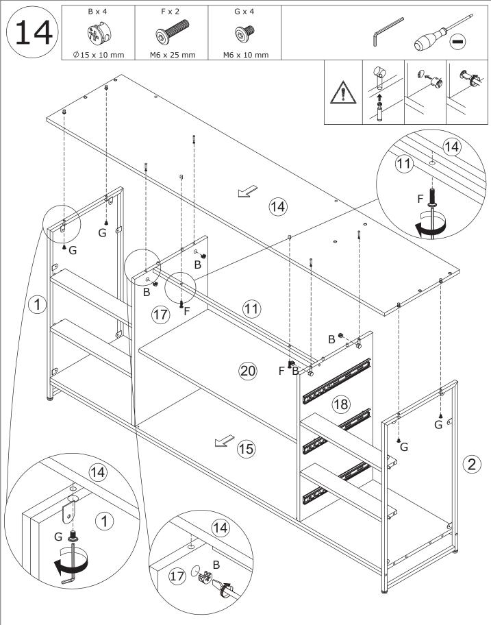
Attach board 14 to the top, add cam lock(B) into board 17 and 18, turn clockwise to tighten as shown.
