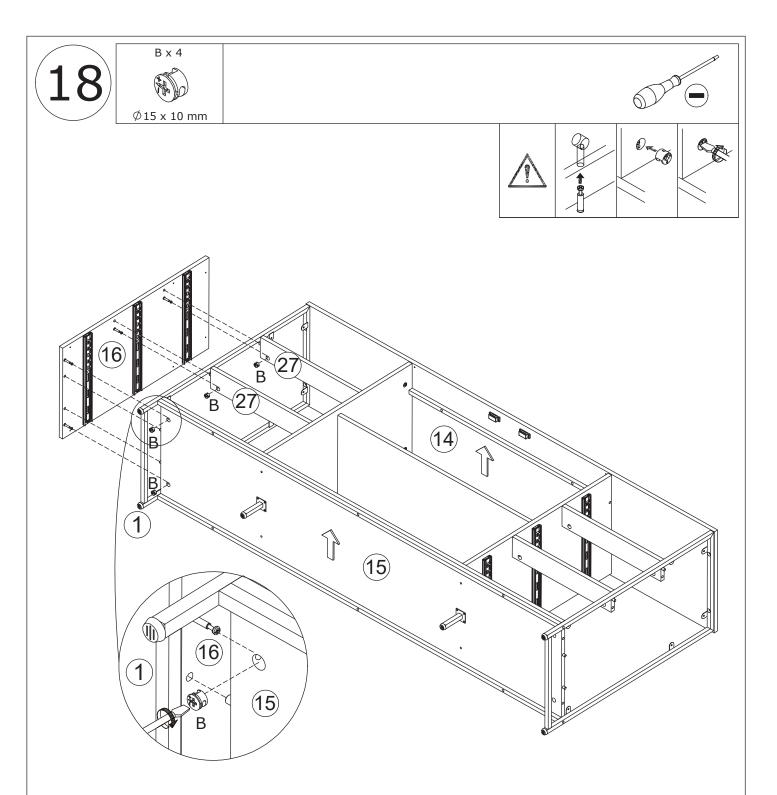
Attach board 16 to board 15 and 27, add cam lock(B) into board 15,27, turn clockwise to tighten as shown.
