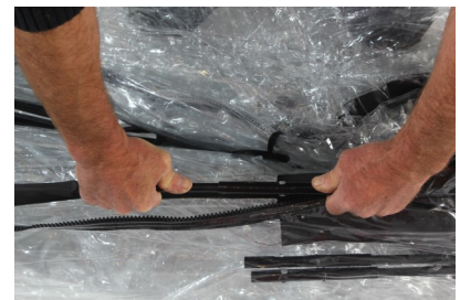
Slide the steel joint over the lower rod
