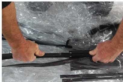
Fit the lower rod into the steel joint
