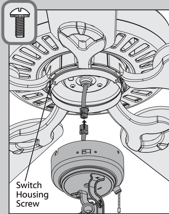
Partially install two of the switch housing screws found in the
