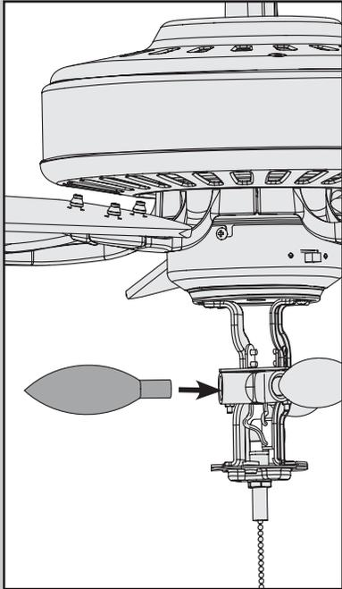
Install a light bulb in each socket.
