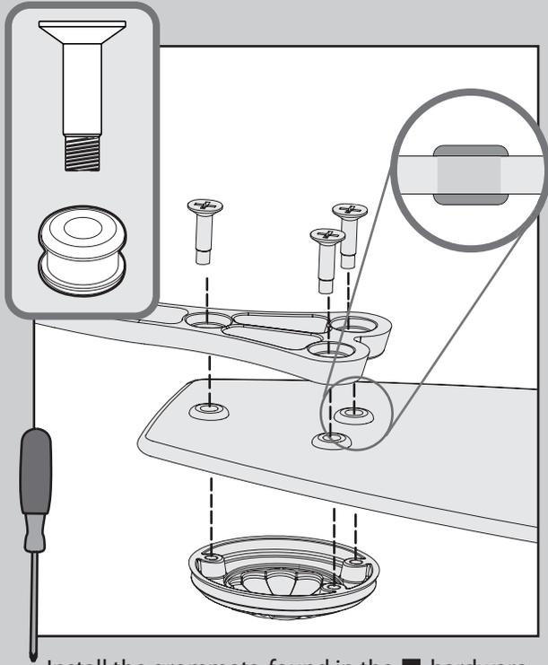
⊗ Install the grommets, found in the ■ hardware bag, in the blades by hand. Place each blade between a blade iron and medallion. Install three blade screws, found in the ▲ hardware bag, to attach the medallion to the blade iron. Repeat for all blades.
