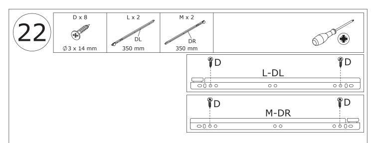
Fix track(L) and (M) to board 17 and 18 with screw(D) as shown.
