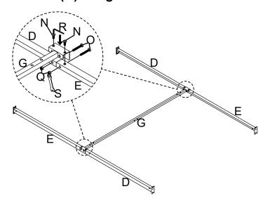
Attach the Rail Support Leg (J) to Center Support Bar (G), and then insert the Bolt (N), turn the L-Allen Key (R) to tighten them.
