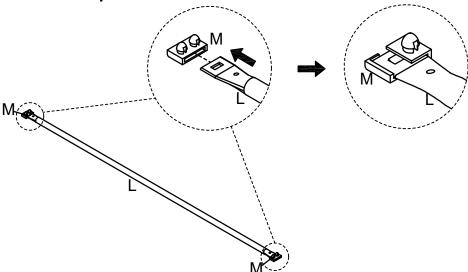
Attached the Slat (L) to rails, put the Slat Connectors (M) into the correct place and press them down.
