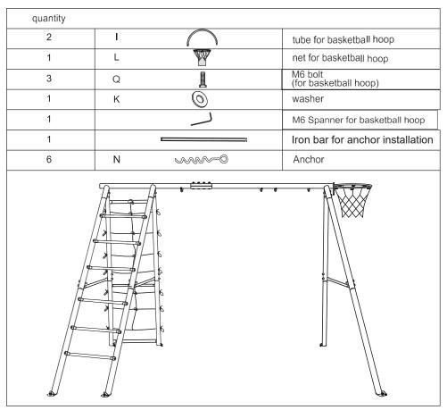
**Step12:** Joint the two I tubes into a circle, and tighten it with M6 screws. (Note: Use M6 spanner to tighten)
