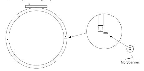
**Step13:** 1. Remove the washer and lock nut on the A2 tube as shown below;
