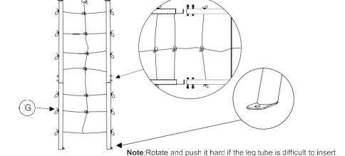
**Step7:** Install three R tubes on the G (Top, Middle, Bottom three positions).
