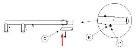
**Step3:** Remove the long bolt on the left, then Put other piece of reinforcing armor on the top of tube.
