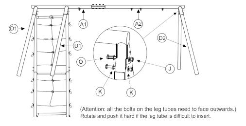
**Step9:** Insert the E1 bottom leg into D1 top leg, E2 into D2, then tighten the screw with a spanner. (Screw the nuts on loosely for 2-3 rounds.DO NOT tighten the nuts in case you need to adjust later.)
