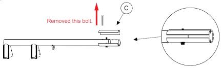
**Step4:** Insert the other A2 tube into the B tube, Make sure these holes are overlapped, then insert a long bolt with washer from the bottom of tube.
