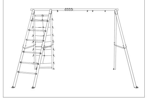
**Step8:** Install the D1 top leg on A1 tube, install D2 top leg on A2 tube, tighten the screw with a spanner. (Screw the nuts on loosely for 2-3 rounds. DO NOT tighten the nuts in case you need to adjust later.)
