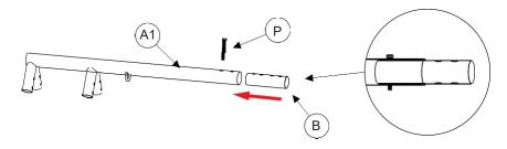
**Step2:** Put a piece of reinforcing armor on the bottom of tube, then insert a long bolt with washer from the bottom of tube. (Attention: All the bolts on the tubes need to face upwards.)
