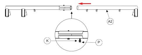
**Step5:** Install the washer and tighten the nut with spanner. (Attention: All the bolts on the tubes need to face upwards.)
