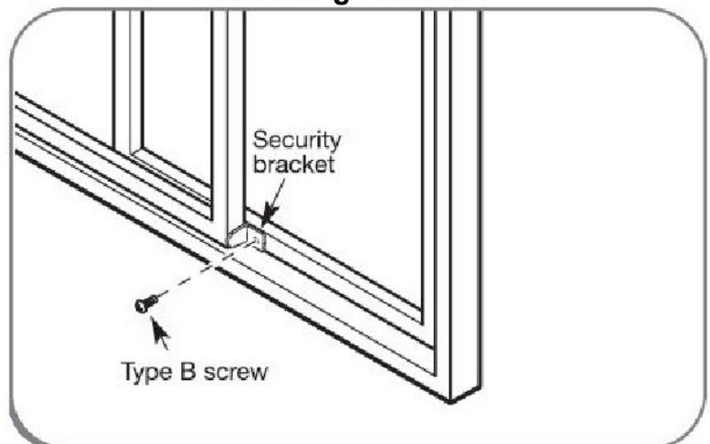
Install the window security bracket with a type B screw as shown.
