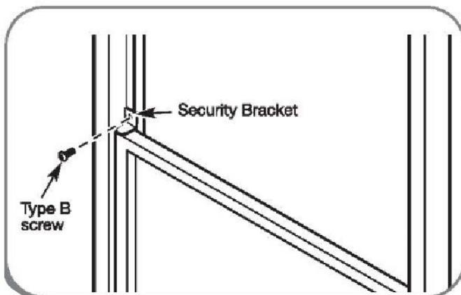
Install the security bracket with a type B screw as shown if you need.
