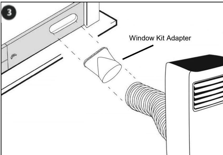
3. Attach the Window Kit Adapter to the Exhaust Hose. Then attach the Window Kit Adapter to the Window Kit panel. Close the window or door tightly.
