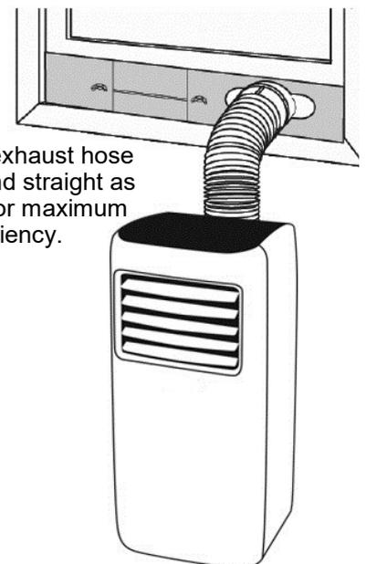
Keep the exhaust hose as short and straight as possible for maximum efficiency.
