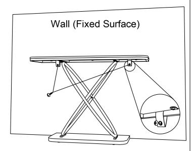
Thread the expansion screw through the round hole the strap and screw it into the hole in the wall.
