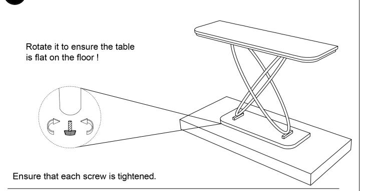
Additional Note About Safety: Bolts may loosen during normal everyday use. They should be periodically inspected and tightened to prevent damage or injury. Always check to be sure that all hardware is kept tightened. Thank you for your purchase.
