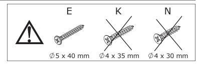
Fix panel 13 and 15 to panel 14 with screw(E) as shown.
