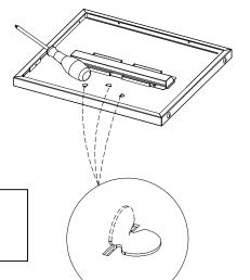
Flat the iron sheet with a screwdriver  $\,$
