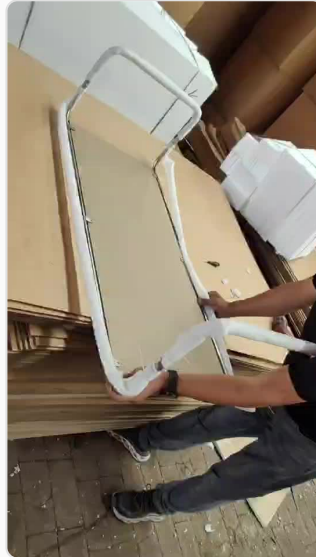
Assembled metal frame ready for tabletop installation
