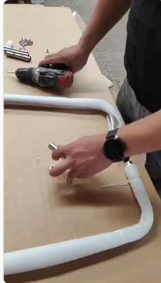
U-shaped side frames with protective foam wrapping
