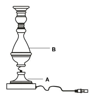
FASTEN SOCKET ASSEMBLY(C) ONTO COLUMN(B).
