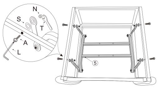
Step 4: Turn chair top upside down on carpet or padded surface and install the swing bracket (5) to bottom tube of the left arm (1) and right arm (2) by using 4 screws(A), 4 flat washers (S), 4 nuts (N), allen wrench (L), and open end wrench (T). PLEASE ATTACH TWO SCREWS IN DIAGONAL POSITION FIRST TO KEEP THE BALANCE, THEN INSTALL THE OTHER TWO SCREWS.
