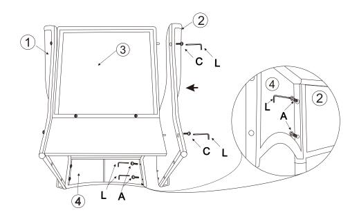
Step 3:Secure right arm (2) to assembled chair back (3) with 2 screws (C) by using allen wrench(L). Then, secure seat panel (4) to assembled right arm (2) with 2 screws (A) by using allen wrench (L). Please tighten all screws now.
