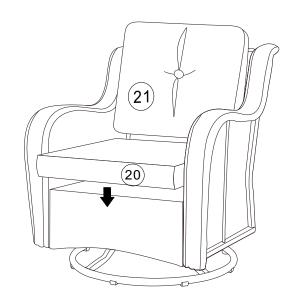
Step 6:Please verify the alignment and adjust, fully tighten all the screws now. Then put seat cushion (20) and back cushion (21) on the chair.
