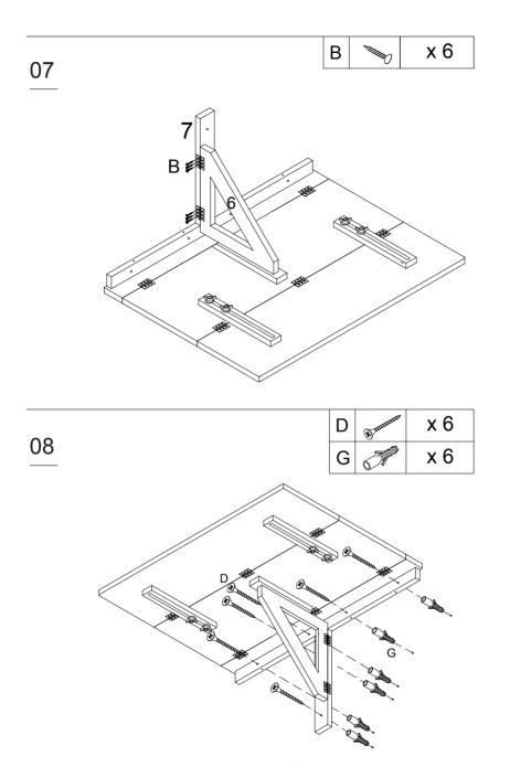
Warning: Ensure that the anchor fits securely in the wall.
