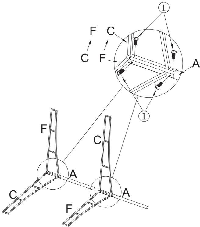
Step 1: Put Part C and Part F together and put Part A in the middle of them, then use four Screw ① to tighten them. Repeat the steps to assemble the other three Part A, Part F and C. Please note: Part C is not the same length as Part F.
