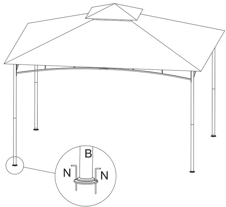
Step 8: Insert the stakes (Part N) on the foot pad to the ground deeply, then you can use the gazebo.
