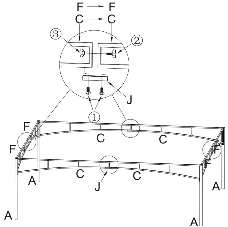
Step 2: Use Nut ③ and Screw ② to attach two Part C (or Part F), and tighten them. Then put one Part J on the bottom side of Part C (or Part F). Use Screw ① to tighten the Part J.
