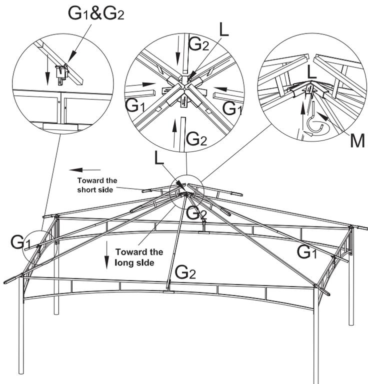
Step 5: Insert Part G1 to the connection part of the two attached Part F. Then Insert Part G2 (the shorter piece) to the connection part of the two attached Part C. Next insert Part E to Part L.
