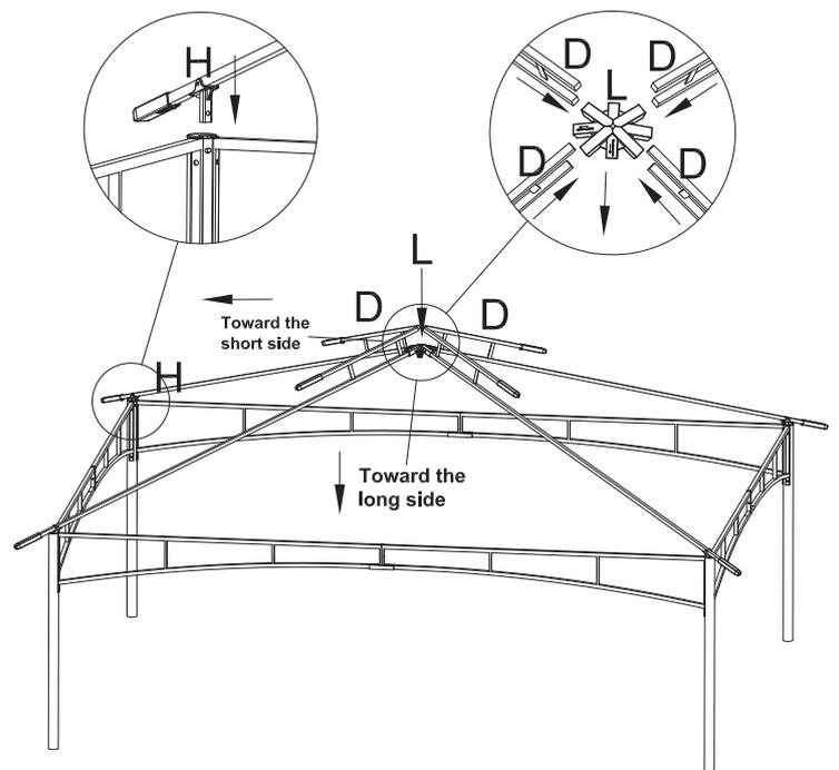
Step 4: Insert four Part H to the four corners of the frame (the top of Part A). Then insert the other side (the bottom side of Part D) to Part L.
