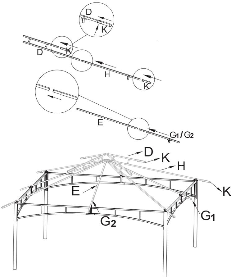
Step 3: Insert the small head of Part H to Part D directly and insert one Part K to the other head of Part H. Then insert one Part K to the short side of Part D. Insert the small head of Part G1 & G2 to Part E. Repeat the steps above to assemble the other Part D, H, K, E and G1 & G2.
