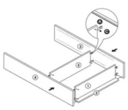
When assemble the A part hardware, do not let the connector pin just sit in the hole, first you need to screw it until its bottom plastic cap is expanded, being fixed in the hole (see below picture).
