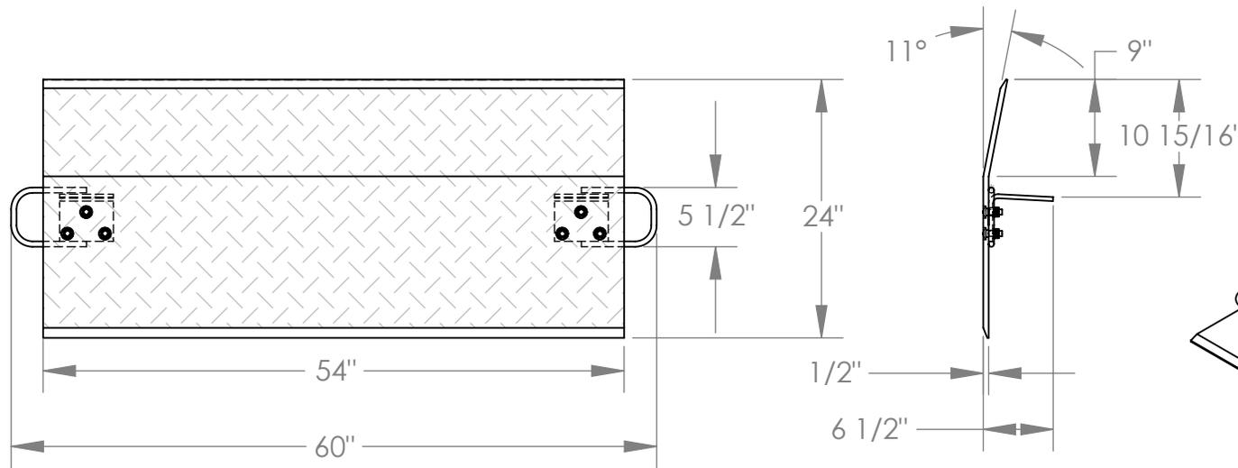
NOTE: BEND OR CROWN IS 11° AND LOCATED 9" FROM EDGE OF DOCKPLATE
