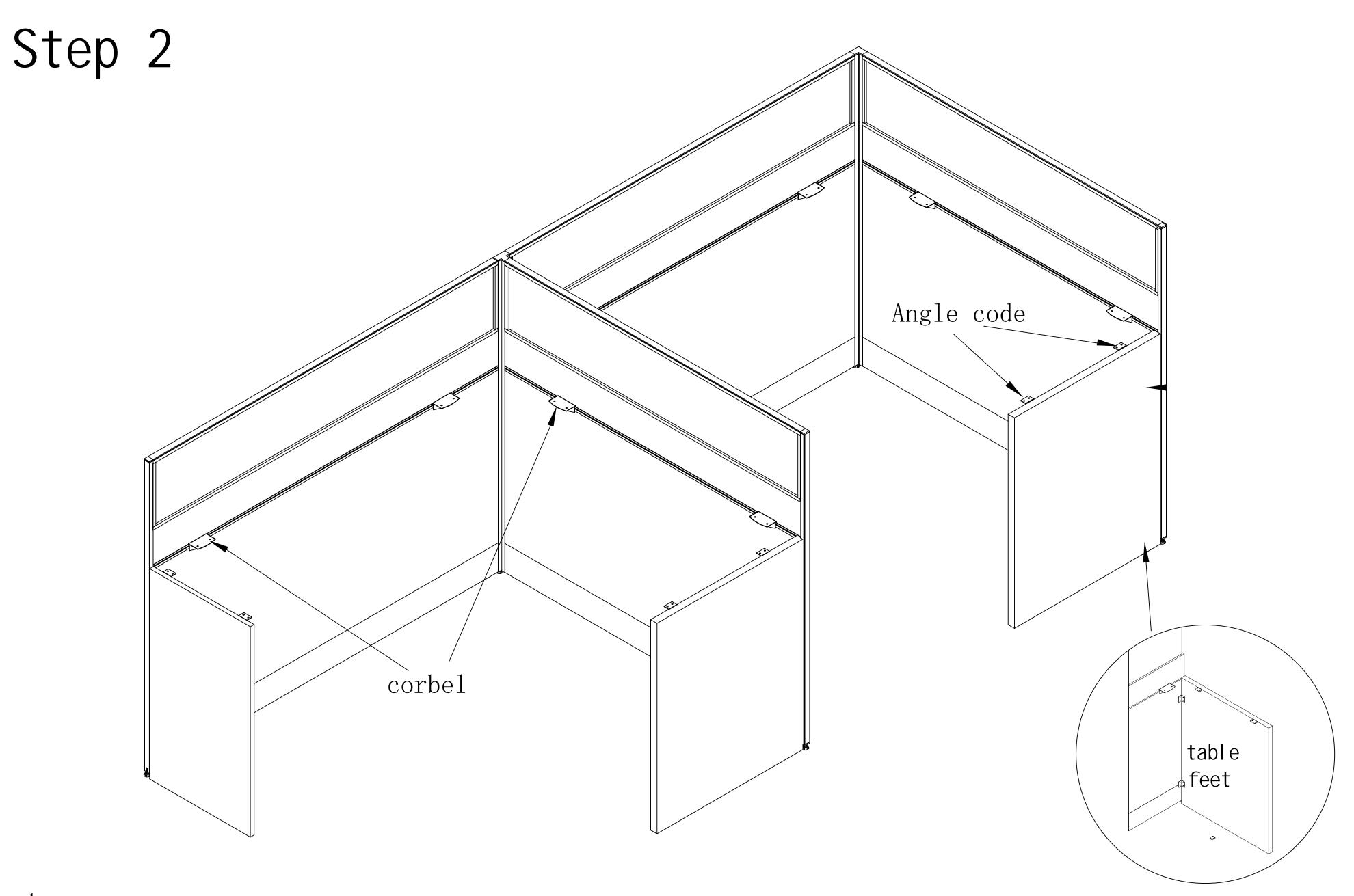
1: Corner code fixing table feet on the screen plate.
