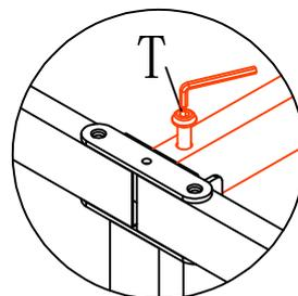
Step2:Joint four corners with screws as shown
