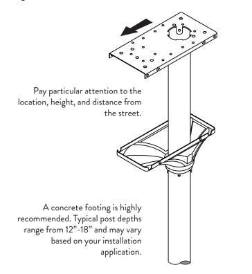
Attach the mailbox to the mounting plate using the 4 large hex bolts, 8 large washers, and 4 large nuts.
