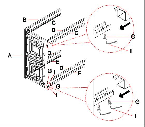
STEP:2. Repeat Step 1 to assembly the assemblied part (B/C/DC/) with another metal frame (A) as diagram shown.
