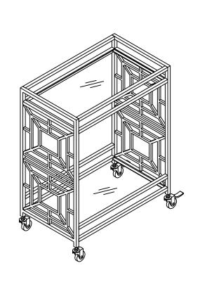
STEP:1. Insert parts"B, C, D, E" into the corresponding male dowels of Metal Frame (A) as diagram shown, then insert the bolt (G) into the corresponding hole of each assemblied part and tighen them an allen wrench accordingly.
