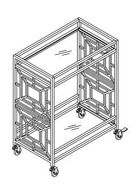
STEP:3. Lay down the assemblied metal frame on a clean and soft surface, then insert the Wheel with brake (J) and Wheel (K) into the bottom of legs as diagram shown, and tighten them with wrench (L).
