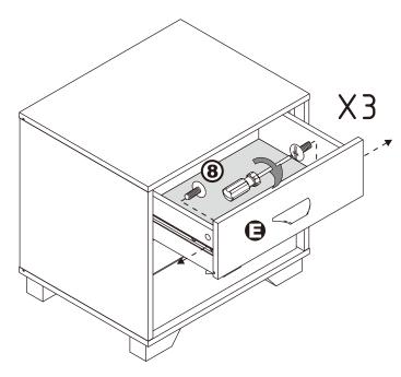
Extend the two outer slides of the runners so that they could align with the sides of the drawer. Make sure the pre-drilled holes from the drawer align with the screw holes of the outer slides.
