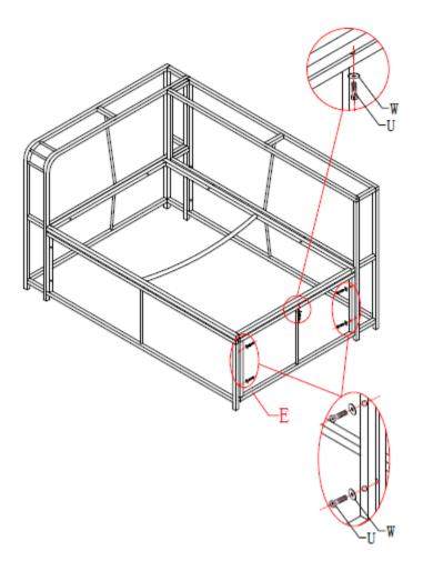
Secure the side piece (E) using screws and washers (W & U).
