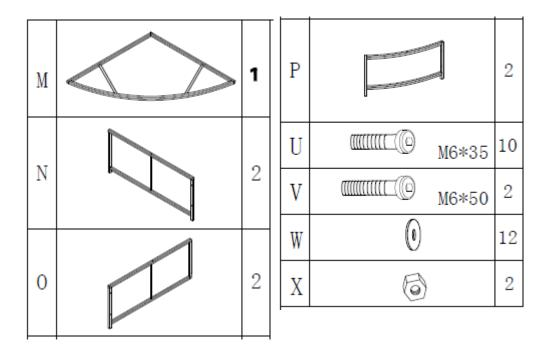
1. Connect pieces M, N and O together using screws and washers (W & U).
