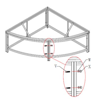
Secure the front pieces together using screws, bolts and washers (V, W & U).
