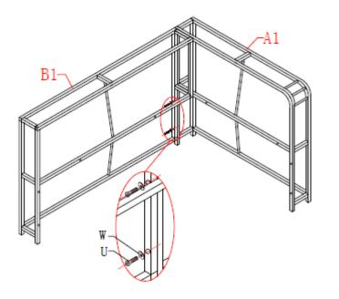
1. Attach B1 to A1 together using screws and washers (W & U).
