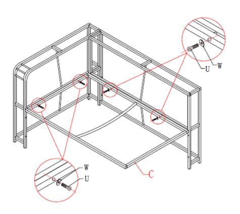
2. Attach the base of the seat (C) using screws and washers (W & U).
