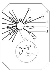
1.Rotate the Arm(J) 5 circles in counter clockwise,then attach the Arm(J) to the Shpere(I) by screwing.
