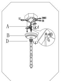
5.Remove the Mounting Bracket(A) from Canopy(B). Fasten the Mounting Bracket(A) to ceiling junction box with screws.
