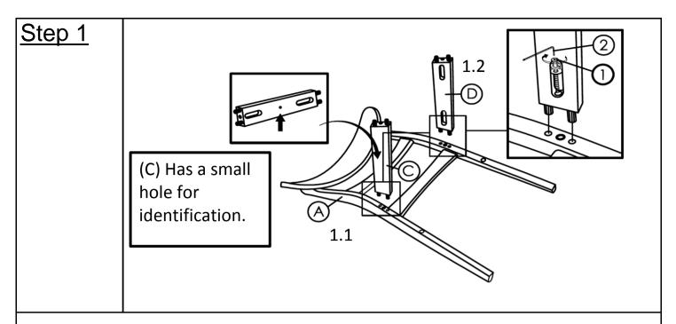
1.1) Insert the Side Stretcher(C) and Side Stretcher(D) into the Chair Back(A) as shown.
