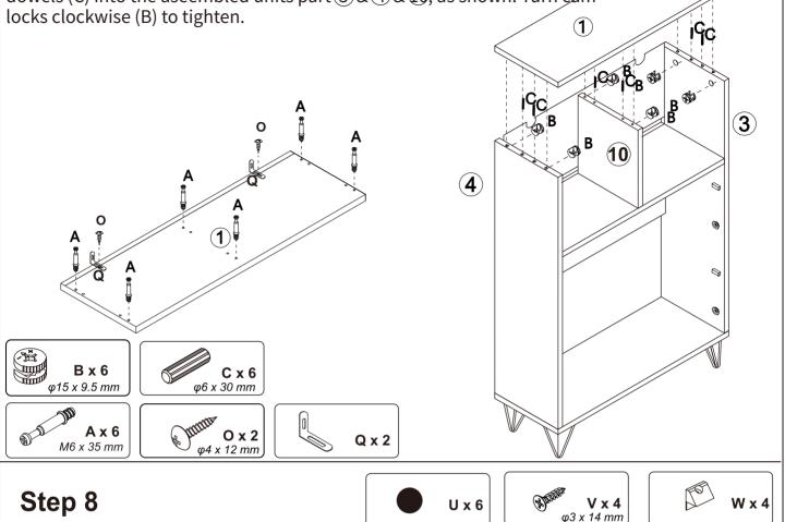
Insert buckle (W) into back slots and fix with screw (V) as shown. Using paster (U) to shield holes.
