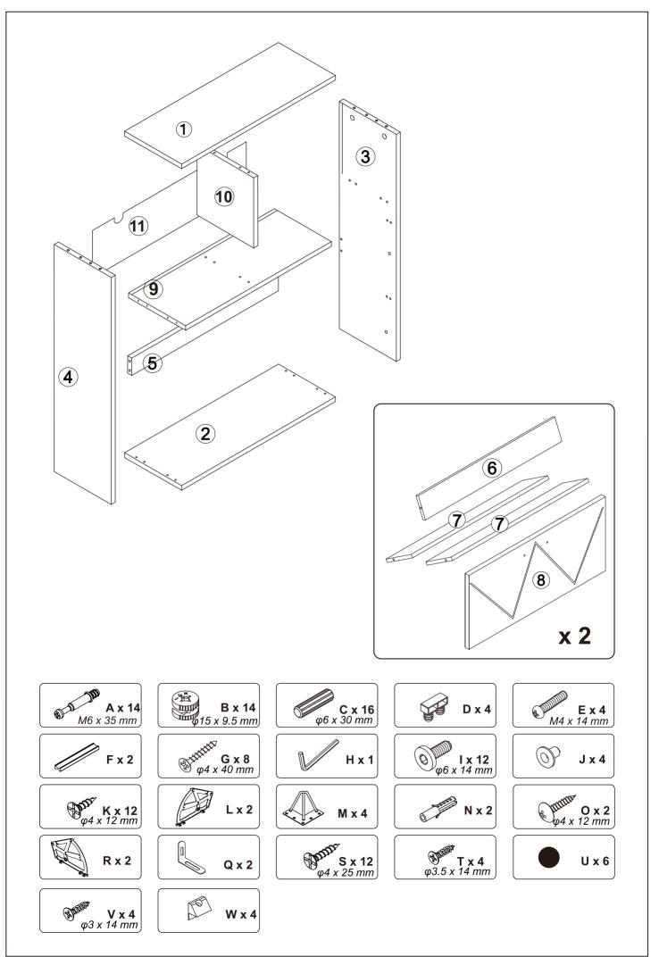
Insert quickfit screws (A) and hardware (D) into corresponding holes in parts (3) (4) as shown.
