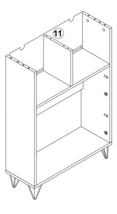
Insert quickfit screws (A) into corresponding holes in part (1), as shown. Fixing Anti-toppling iron sheets (Q) with screws (O). Then Insert wooden dowels (C) into the aseembled units part (3) & (4) & (10), as shown. Turn carn locks clockwise (B) to tighten.
