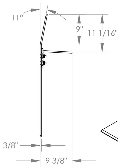
NOTE: BEND OR CROWN IS 11° AND LOCATED 9" FROM EDGE OF DOCKPLATE
