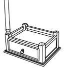
**STEP 2:** Slightly screw one leg to the bottom of the table-top and gently tighten the leg. Do not screw the leg too tight.
