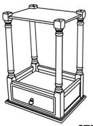
**STEP 4:** Put the bottom shelf over the end of the four legs, slightly adjust the wooden legs so the screw holes on the legs are lined with the holes on the bottom shelf.
