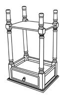
**STEP 6:** Slightly screw the other three feet through the bottom shelf to connect with the wooden legs.
