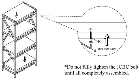
Attach back rail (5,6,7) to side rail (2,3), JCBC screw (B), tighten by using allen-key (A). Secure with bracket-tip restraint (C).
