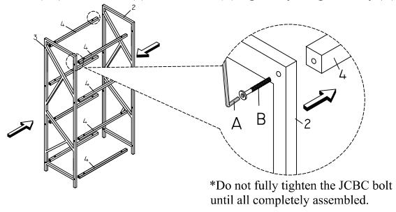
Attach fixed shelf (1) to metal rail (4), JCBC screw (B), tighten by using allen-key (A).
