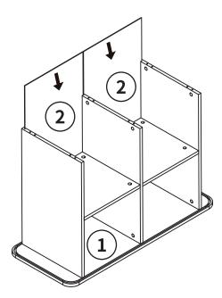
Insert Board (2) into the grooves on Board (1).
