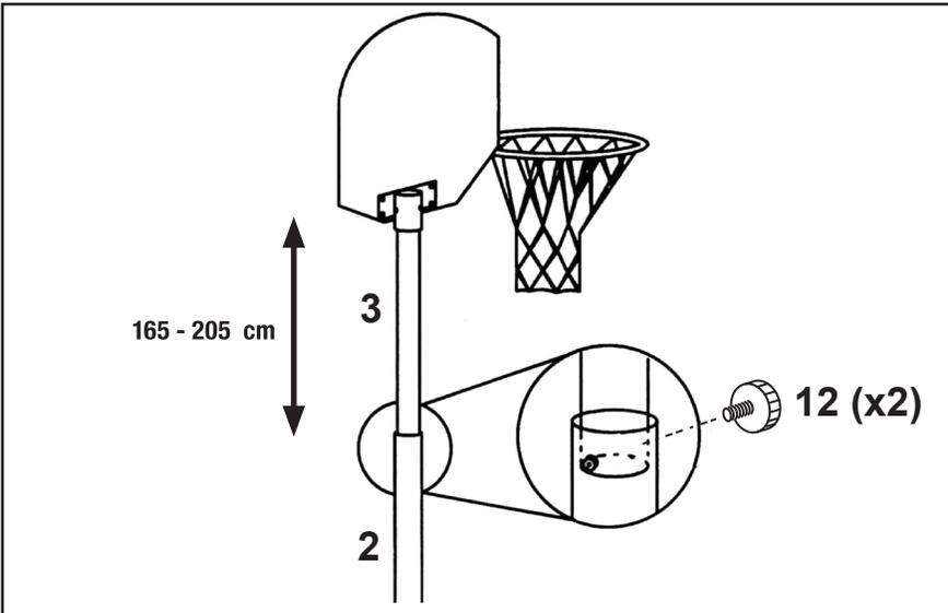
Loosen Knob Bolts (12) to adjust height. Tighten to keep in place
