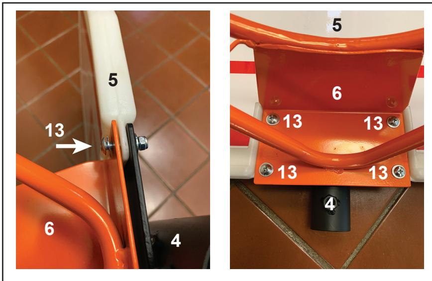
Use four Rim Bolt Sets (13) to attach Basketball Rim (6), from front side, thru holes in Backboard (5) and to Connecting Plate (4), on back side. *Note: Use Washers (13) on both sides.* Tighten bolts (13)
